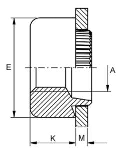
Female thread A = M2,5Height K = 3.0Outer diameter E = 6.0Plate thickness = 3.2 to 3.4
